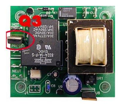
There is an extremely rare case where the heat can continually rise well beyond the temperature setting on a Digital Knight heat press. In this case, remove Q3 before resorting to simply replacing the power board.
