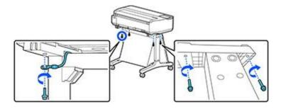
If your stand includes thumbscrews, insert 4 thumbscrews (2 on each side) into the bottom of the
