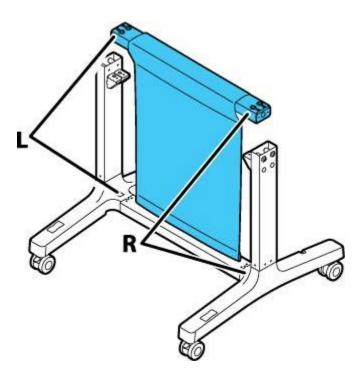
6. Insert 4 screws (2 on each side) into the holes on the paper basket bar to secure it to the legs.
