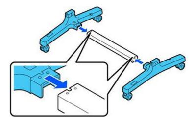
2. Use the Allen wrench to insert 8 screws (four on each side) into the holes on the support brace and leg bases as shown.
