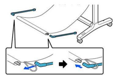
11. Insert the ends of the paper basket support rods into the holes on the leg bases.
