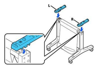
8. Insert 4 screws into 4 screw holders (2 on each side) and insert them into the holes on the legs to secure the mounting brackets.
