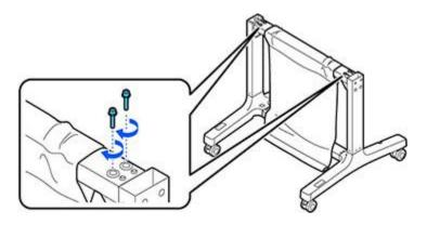
7. Make sure the L and R stickers on the mounting brackets are correctly oriented with the left and right legs and attach them as shown.
