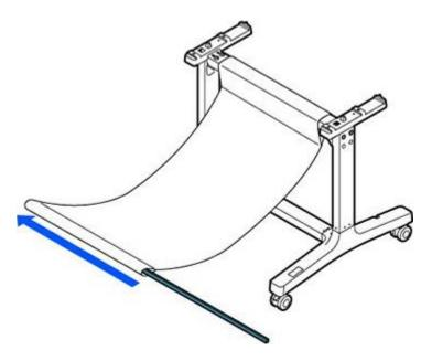
10. Insert the top of the paper basket support rods through the loops on the paper basket cloth and attach them to the paper basket rods.
