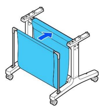
13. On the back of the paper basket and stand, attach the loops on the paper basket cloth to the hooks on the leg bases as shown.
