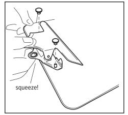
**Step 2:** Hold open the clip and apply over the rivets. This will take a bit of force. Attach top rivets to the bottom rivet shafts. Once rivets are seated in place, you can release the clip and grab the hammer to finish securing the rivets.
