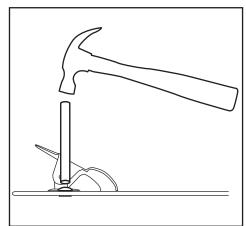
**Step 3:** Use the hammer and drill bit punch (or bolt) to tap the rivet into place.
