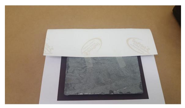
Center the substrate on your image and fold over one edge and use two pieces of tape to make sure the paper will not shift
